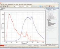
processing, other features include automatic dark removal, spectrum smoothing, and manual/auto baseline correction. SDK with demo code is available as additional option.
