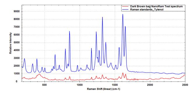
The intensity of the measurement is much lower than that from a transparent bag, but it still gives adequate Raman signature to find the correct match within the library.
