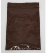
This technical note is to demonstrate the ability of the NanoRam<sup>®</sup> (785 nm laser excitation) for material identification through dark brown plastic bags. Tests have been done for material identification test directly from outside dark brown polyvinyl bag using NanoRam.
