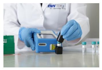
reproducibility. The focal point of the measurement is a few millimeters from the vial wall, providing a spectrum of the material inside the container and minimizing glass contribution (clear or brown).
