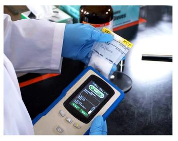
common and versatile of all accessories. Simply press the sample against the accessory and hold it in contact until the end of the data acquisition.
