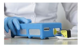
For hands-free measurement of samples on a surface, the **Right Angle Adaptor** is an accessory that facilitates measurements at a 90° angle, allowing the NanoRam to be placed on a surface (such as a lab bench) and the measurement to be made without the need for holding the sample or the unit during the course of the analysis. Samples can be in transparent sample bags or measured directly. The data are obtained approximately 1mm below the contact
