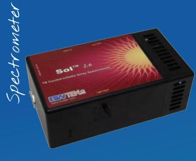
The **Sol**<sup>imesilon</sup> **2.6 (BTC263E)** is a high performance linear InGaAs array spectrometer featuring 256 pixels, high throughput ,and large dynamic range, with TE-cooling down to -15° C via a built-in 3-stage cooler.
