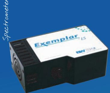
The Exemplar® Plus LS (BTC645N) is a high-performance smart spectrometer utilizing an aberration-corrected concave holographic grating to effectively eliminate stray light. It features a highly sensitive TE-cooled back-thinned (BT) CCD detector which is linearly summed for high dynamic range. Its long focal length, coupled with a high quantum efficiency detector, provides superior data quality over the entire 180 - 1100 nm spectral range.
